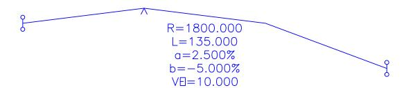
Crest curve created with maximum horizontal step size of 25, resulting in a smoother curve than above
