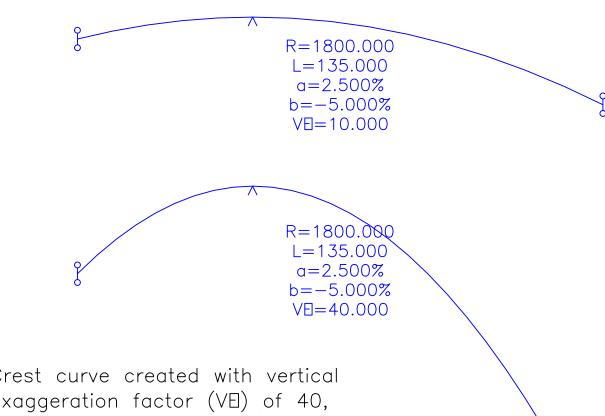
Crest curve created with vertical exaggeration factor (VE) of 40, resulting in a curve which no longer presents a practical representation of the curve
