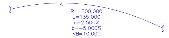
Note that the horizontal step size drawn will be rounded down to fit the overall curve length and also to ensure the minimum or maximum level is drawn in the curve. This can result in slightly different steps sizes either side of the minimum or maximum level point
