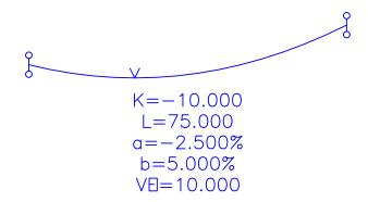
Typical sag curve with K value entered instead of radius value (K=-10 is equivalent to R=-1000)
