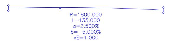
Crest curve created with vertical exaggeration factor (VE) of 10, resulting in a curve which is easier to visualise
