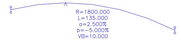
Crest curve created with maximum horizontal step size of 10, resulting in a smooth curve
