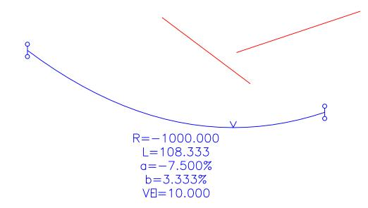
Crest curve fitted to two lines used as references for start and end gradients
